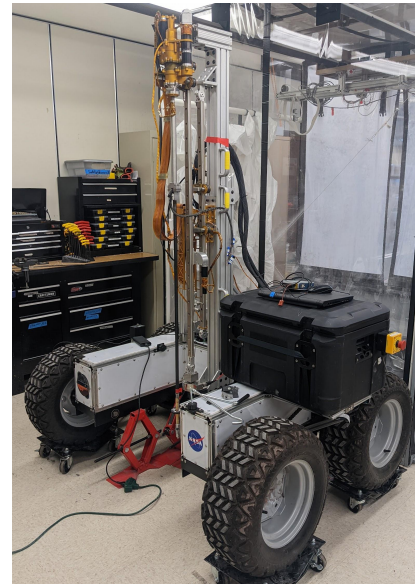
Figure 1: Modified TRIDENT z-stage integrated with HOPLITE rover chassis.
